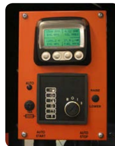
PrimeGuard is available as an option on all CD and HL series Dri-Prime pumps with diesel engine ratings greater than 140 kW.
